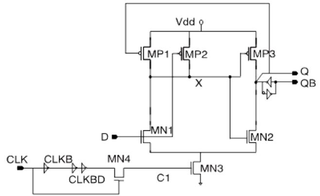
Fig.2 Modified Hybrid Latch Flip-flop
