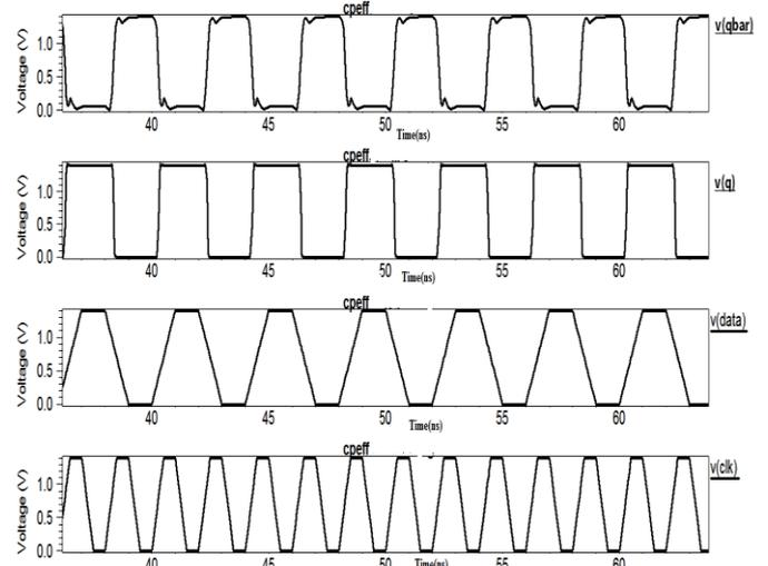
Fig.6 Simulated waveform for 90nm CPEFF design
