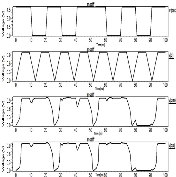
Fig.4 Simulated waveform for 90nm master slave D-flip-flop design
