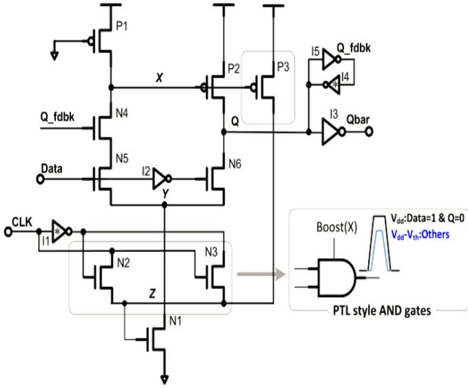
Fig.3 Conditional pulse enhancement flip-flop
