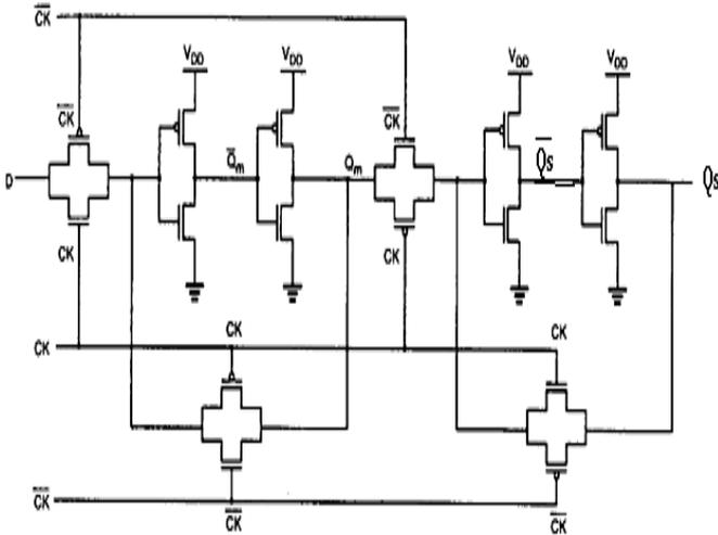
Fig.1 CMOS negative edge triggered master-slave D flip-flop using transmission gate
