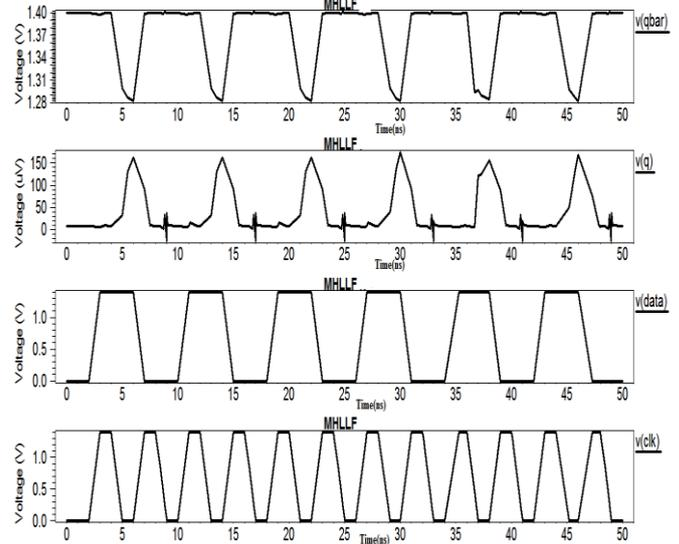
Fig.5 Simulated waveform for 90nm MHLFF design
