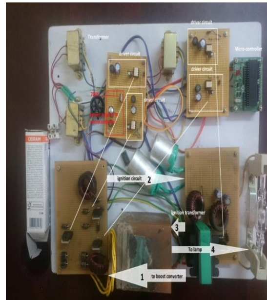
Fig 10. Hardware prototype of electronic ballast for 70watt OSRAM lamp
