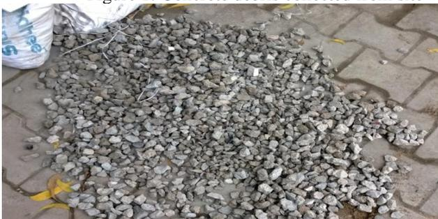
Figure 2: Generated RCA from debris
