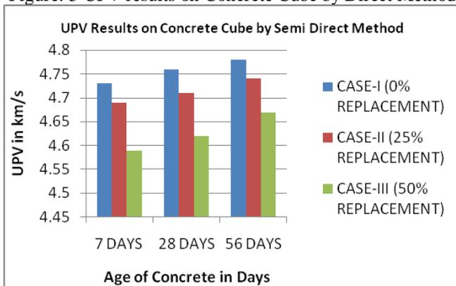
Figure: 6 UPV results on Concrete Cube by Semidirect Method
