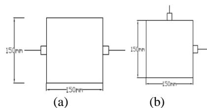
Figure: 4 UPV measurements on concrete Cube by (a) Direct Method (b) Semidirect Method
