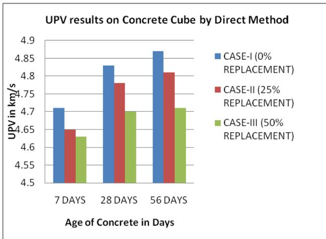
Figure: 5 UPV results on Concrete Cube by Direct Method
