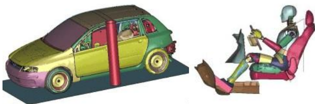
Fig.9. Rigid Pole and Dummy representation for side impact
