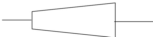
FIGURE:1 Tepered Microstrip Transmission Line
