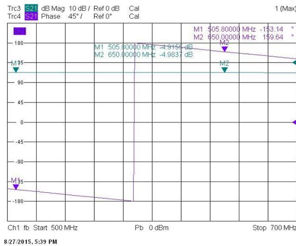
FIGURE 6 VNA Measurements of WB 2-Way Tapered Microstrip Line Power Divider
