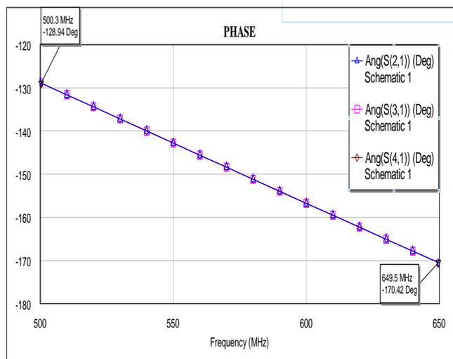
FIGURE 4 Phase of WB 3-Way Tapered Microstrip Line Power Divider
