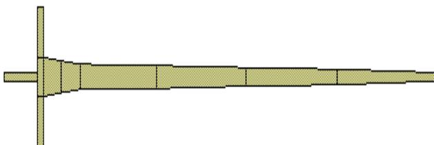
FIGURE 2 Layout Of WB 3-Way Tapered Microstrip Line Power Divider
