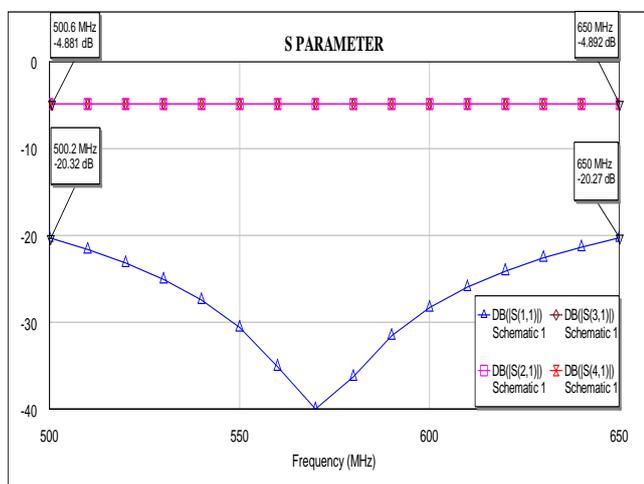
FIGURE 3 Graph Of Wb 3-Way Tapered Microstrip Line Power Divider
