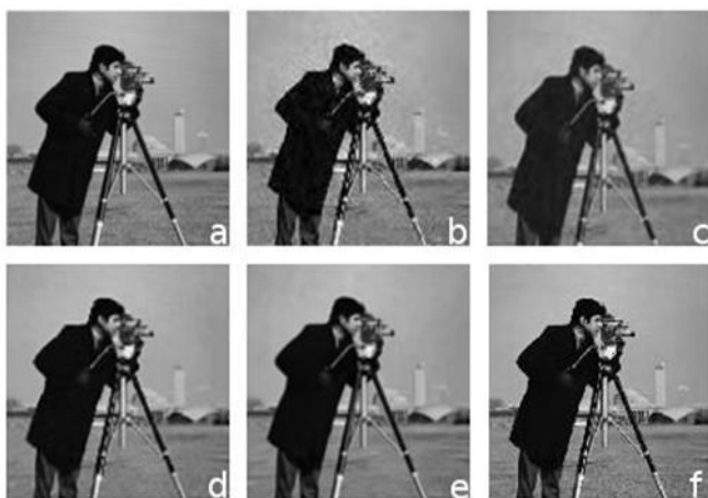
Fig. 5. The denoising results of Cameraman by different schemes. (a) Noiseless Cameraman; denoised images by methods (b)[3,6]; (c) [10]; (d) [24]; (e) [23]; and (f) the proposed PCA-SPT method.
