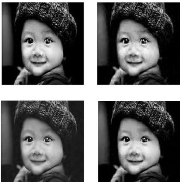
Fig. 3. (a) Original image Baby; (b) noisy image (PSNR= 28.1 dB); (c) denoised image after the first stage of the proposed method (PSNR= 34.6 dB) and (d) denoised image after the second stage of the proposed method (PSNR=35.2 dB). We see that the visual quality is much improved after the second stage refinement.
