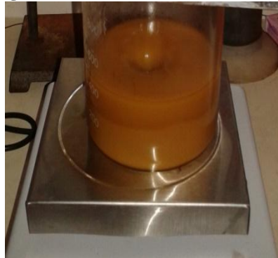
Figure No 2: Reaction of Mixture on Magnetic Stirrer
