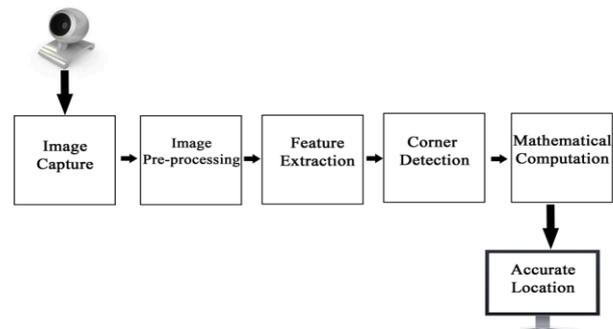
Fig. 1 HCI System Architecture
