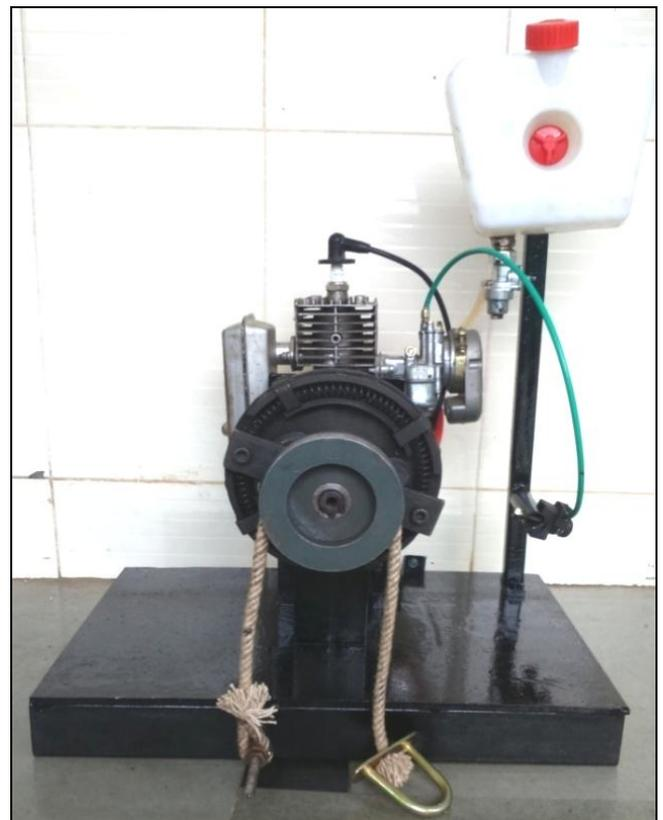
Fig. 9 Actual setup of dual mass flywheel test rig
