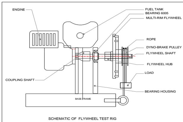
Fig. 7 Schematic of conventional flywheel test rig
