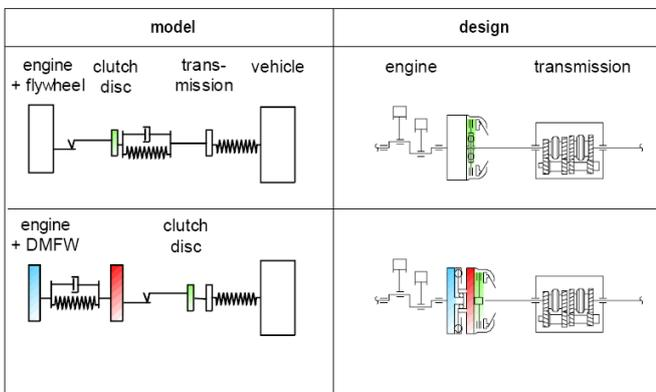
Fig. 3 Principle of the dual mass flywheel [2]
