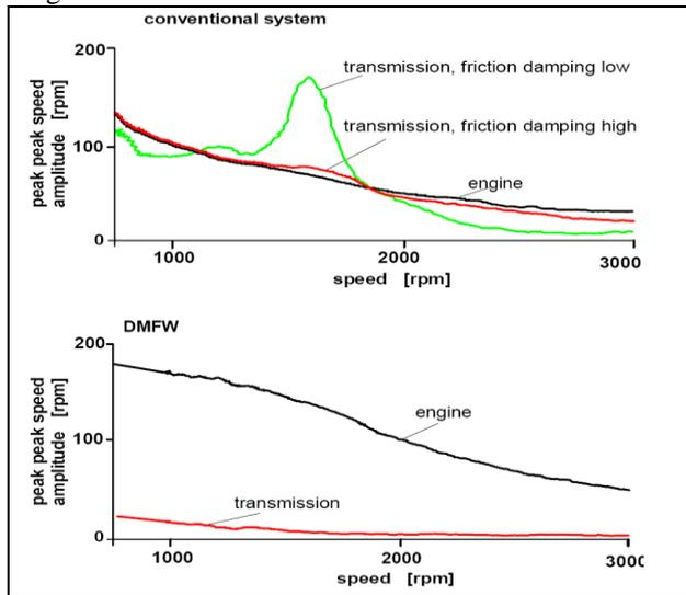
Fig. 2 Torsional vibration isolation with conventional clutch disc and dual mass flywheel [2]
