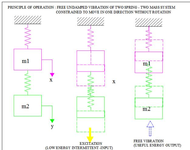
Fig. 4 Graphical Model of spring mass flywheel system
