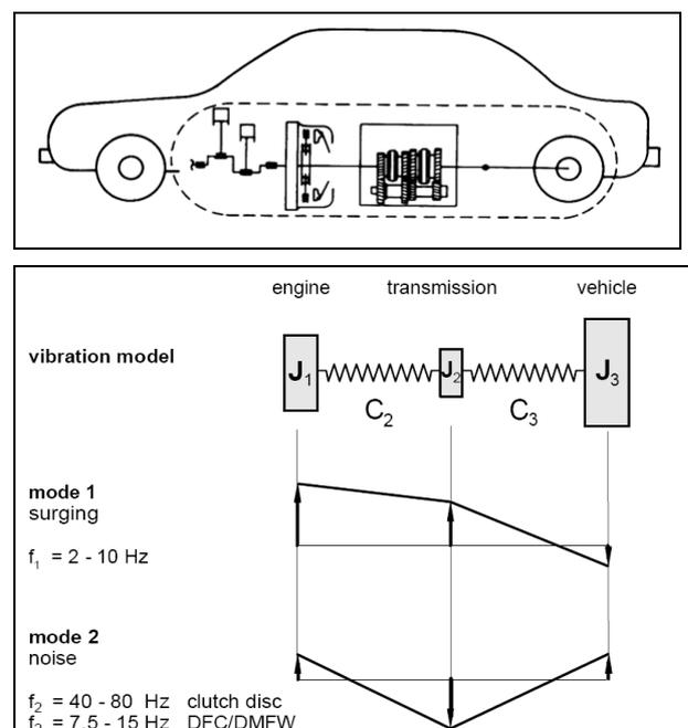
Fig. 1 Vehicle drive train with vibration modes<sup>[1]</sup>
