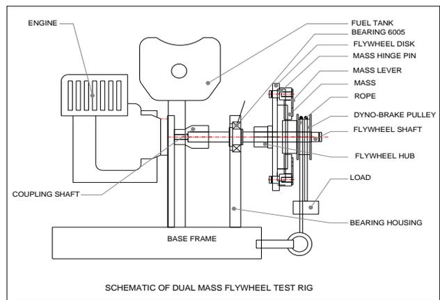
Fig. 8 Schematic of dual mass flywheel test rig
