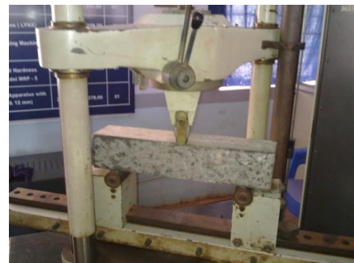
Figure 5: Flexural Test on Beam
