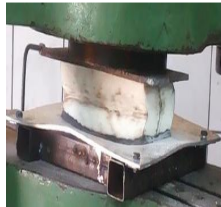
Figure 9: IMPACT ATTENUATOR AFTER TESTING
