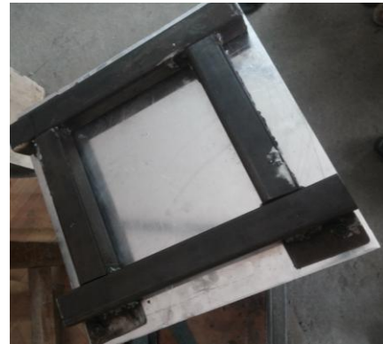
Figure 7: FIXTURE FOR IMPACT ATTENUATOR TESTING
