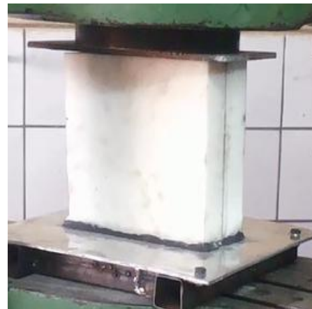
Figure 8: IMPACT ATTENUATOR DURING TESTING
