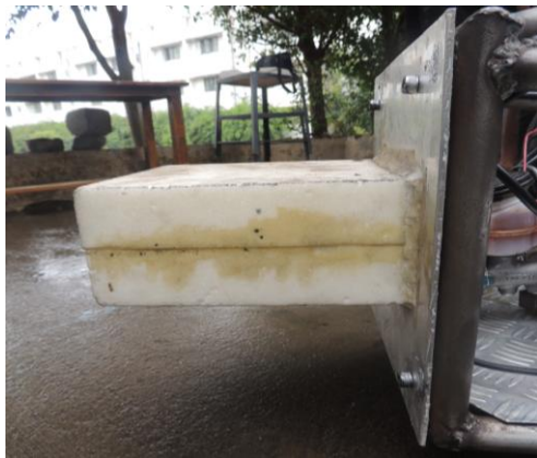
Figure 6 : ACTUAL IMPACT ATTENUATOR MOUNTING.
