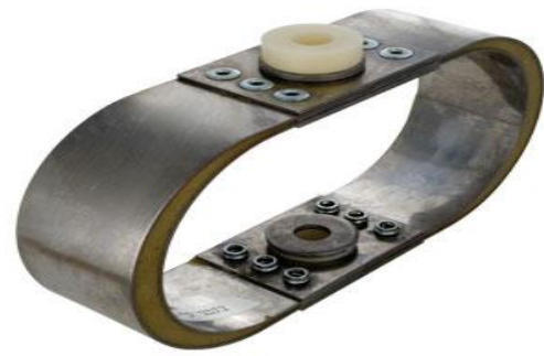
Fig 2: Elliptic Leaf Spring Mounts from Advanced Anti-vibration Components. The static loads for these springs range from 10 to 500 Kg per mount and have a natural frequency of 5~10 Hz (vibrationmounts.com).
