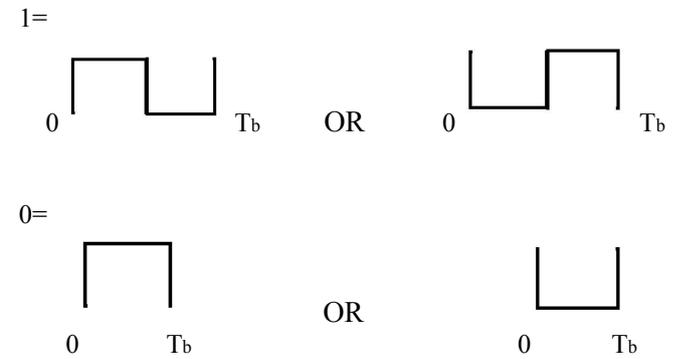
Fig.2 Representation of '1' and '0' bits in Biphase-M
