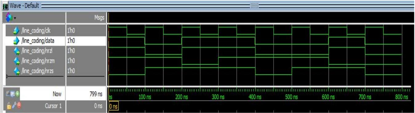
Fig.4 Screenshot of Waveforms after Simulating NRZ Line Coding schemes
