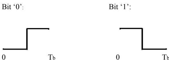
Fig.1 Representation of '1' and '0' bits in Biphase-L
