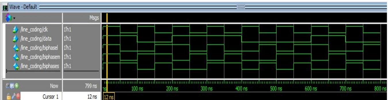
Fig. 6 Screenshot of Waveforms after simulating Biphase Line Coding schemes
