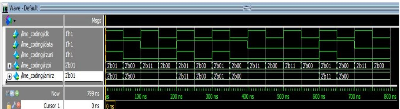
Fig. 5 Screenshot of Waveforms after simulating RZ Line Coding schemes
