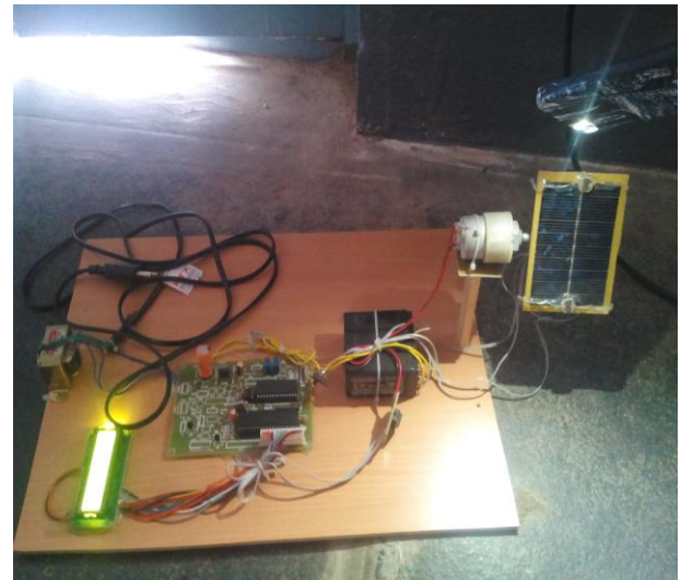
Figure 4. Real time DUAL-DIRECTION SUNTRACKING SOLAR SYSTEM
