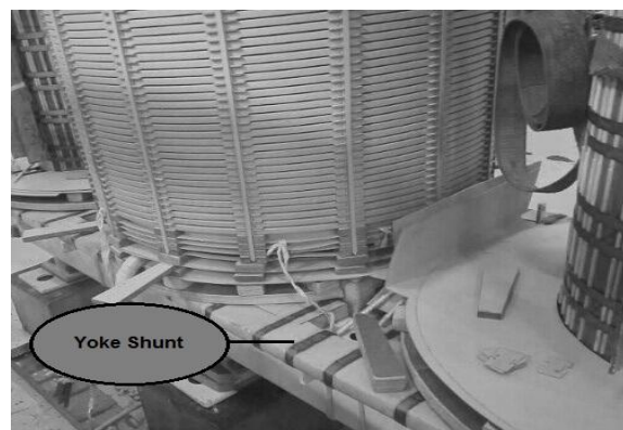
Figure: 6 Yoke shunting for stray reduction
