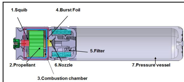
Fig 2.Components of an Inflator
