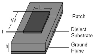
Fig. 2: Geometry of Microstrip antenna
