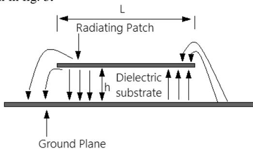
Fig. 3: Radiation in antenna
