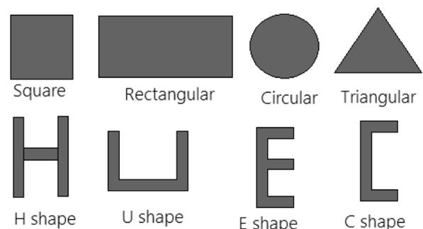
Fig. 1: Different shapes of microstrip patch antenna
