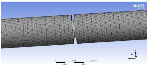
Fig. 3 Meshing of orifice meter
