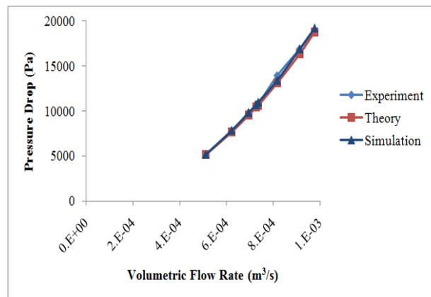
Fig. 6 Comparison of Pressure drop from Experiment, Theory and Simulation
