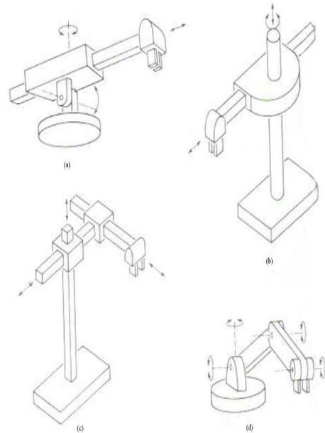
joint motions associated with these two categories are sometimes referred to by the term “degrees Of freedom”, and a typical industrial robot is equipped with 4 to 6 degrees of freedom. Here we use Robotic Arm for Pick and Place purpose.
