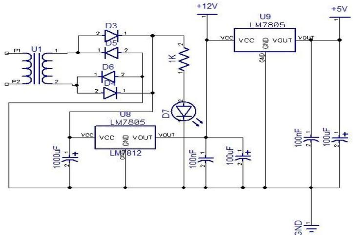
Fig. 8: Circuit diagram of the power supply module
