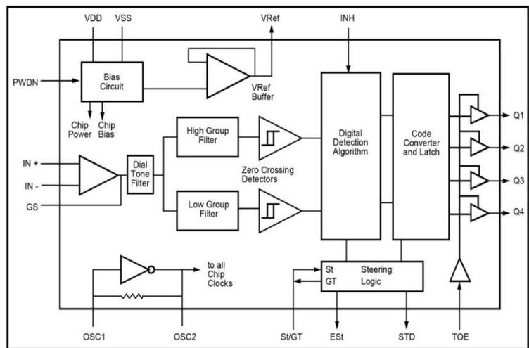
**Fig.4:** Functional block diagram of a DTMF tone decoder chip
