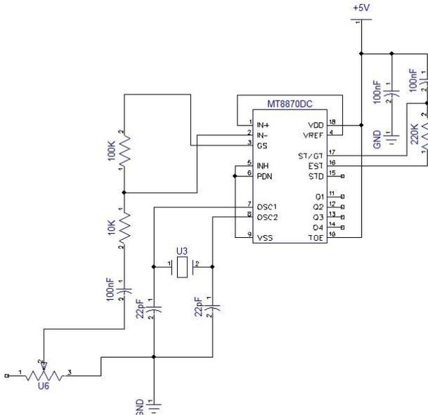
Fig. 6: Circuit diagram of the DTMF decoder module
