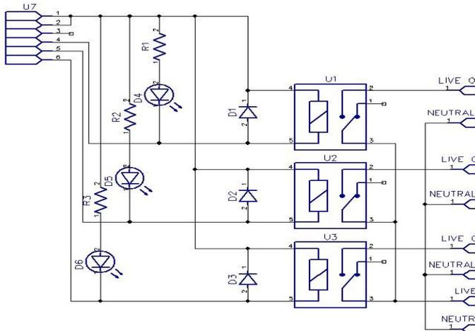
Fig.7: Circuit diagram of the output Relay Module
