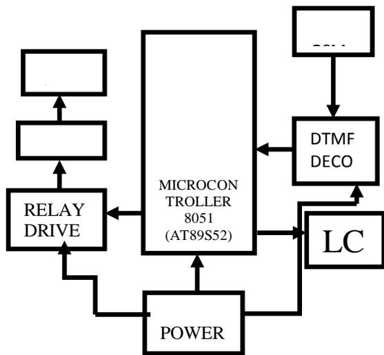
**Fig.1** Block diagram of GSM-based multi-purpose measuring device
