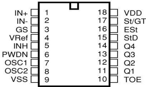
Fig.5: Pin configuration of MT8870 DTMF decoder
