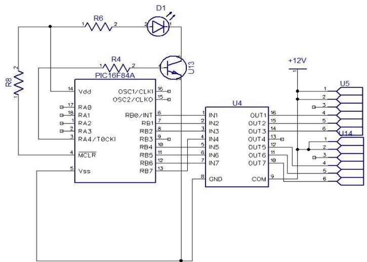
**Fig.3:** Circuit diagram of the output relay module
