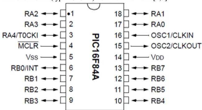
**Fig. 2:** Pin out diagram of PIC Microcontroller (type 16F84A)
