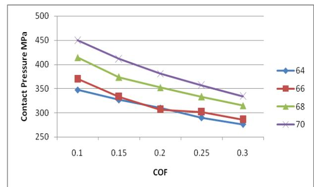
Figure 2 Variation of contact pressure with flank angle
