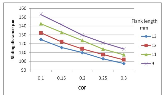
Figure 3 Variation of sliding distance with flank length
