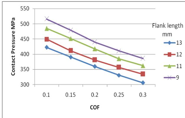
Figure 4 Variation of contact pressure with flank length
