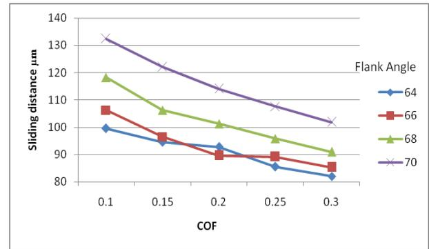
Figure 1 Variation of sliding distance with flank angle
