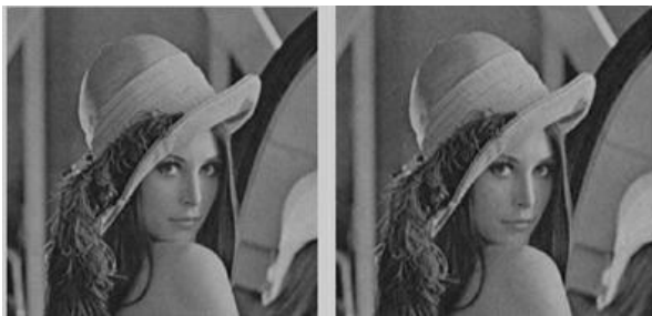
Fig. 5 Reconstructed image (a) PSNR=37.78 Compression ratio without using Huffman coding is 5 and with Huffman coding 42.54 for \lambda = -20 (b) PSNR=26.72 Compression ratio without using Huffman coding is 6 and with Huffman coding 28.91 for \lambda = -50
