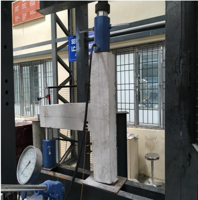
Figure2: Test Setup for beam column Joint III. EXPERIMENTAL PROCEDURE
