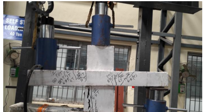
Figure 5: Failure pattern of Beam-Column joint
