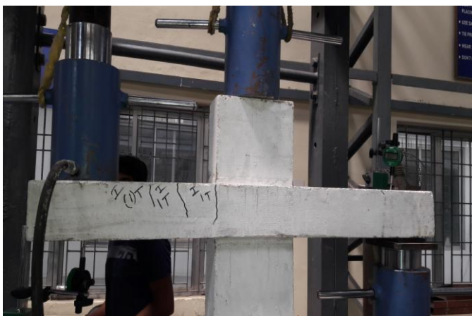
Figure 4: Test setup of wide Beam-Narrow Column joint
