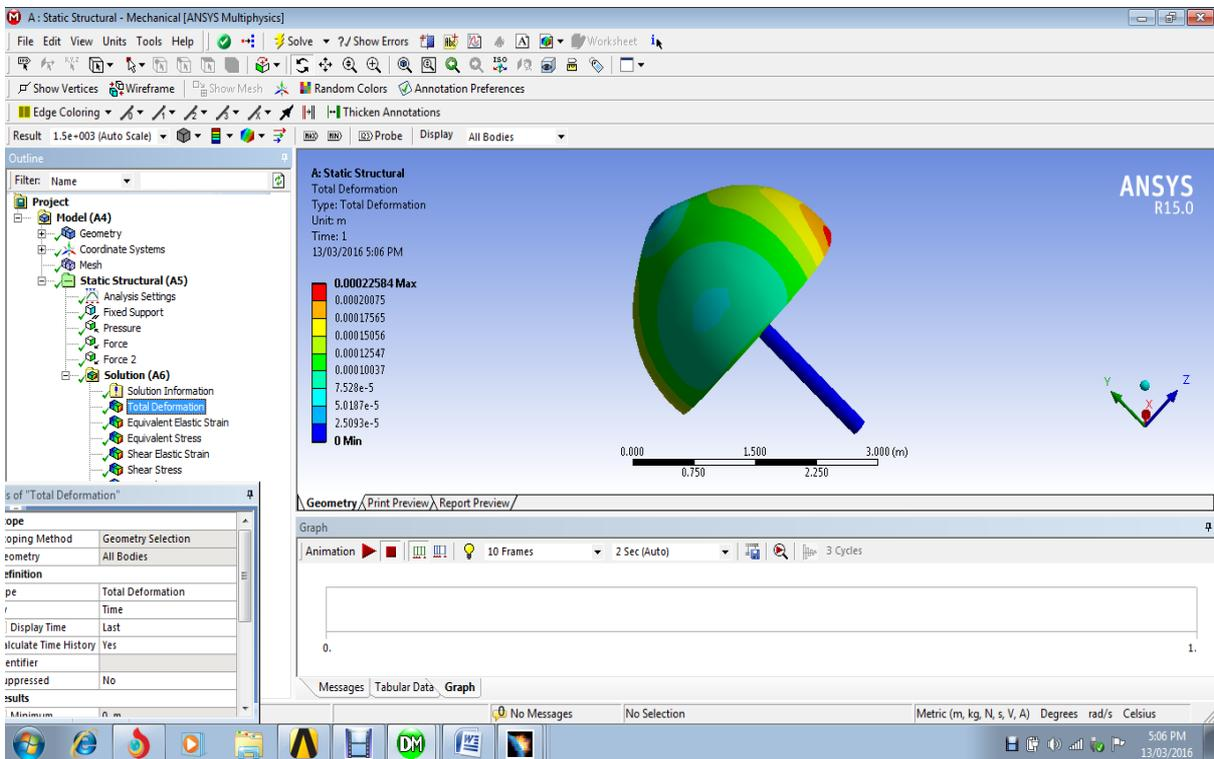
Figure 3: Total Deformation of the structure
