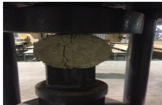
Figure-3 Split tensile test
