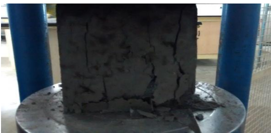
Figure-3 Compressive strength test
