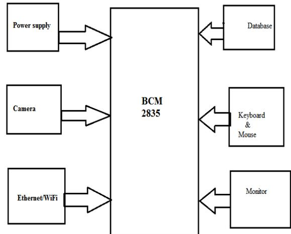
**Fig 1. BLOCK DIAGRAM of BCM 2835**
