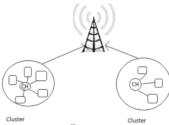
Figure 2: Cluster-Based Routing In WSN
