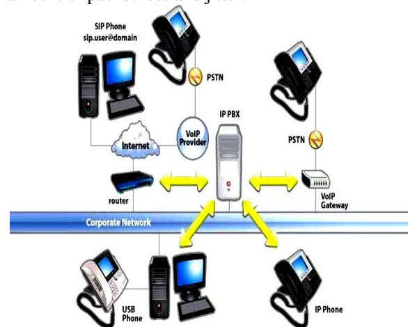
Figure 1: Structure of Voice over Internet Protocol (VOIP)
