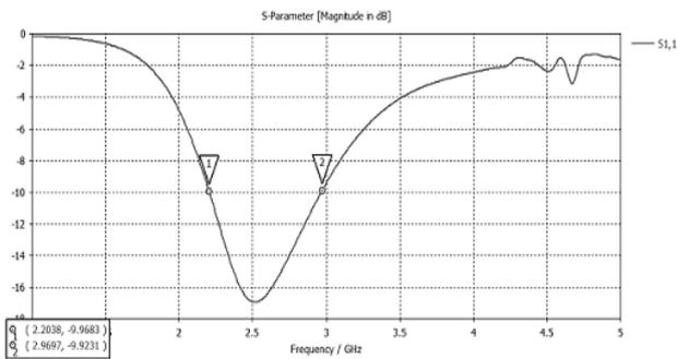
Fig.6 . Return loss of simple patch loaded with srr resonating at 2.5ghz enhanced bandwidth.
