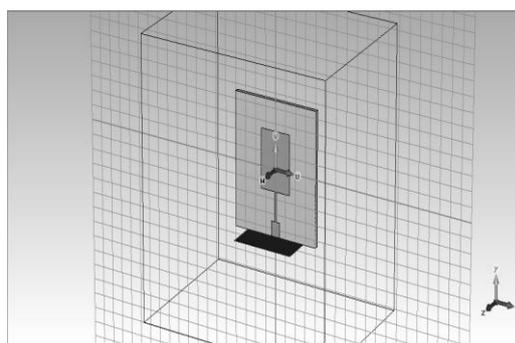
Fig.4 . Conventional Rectangular Patch antenna
