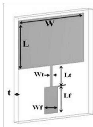
Fig.1. Patch antenna design
