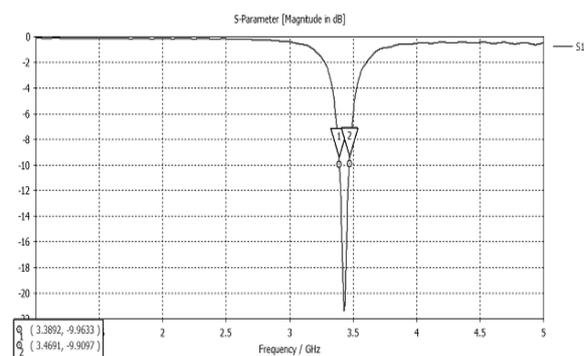
Fig.5. Return loss of simple patch resonating at 3.428ghz
