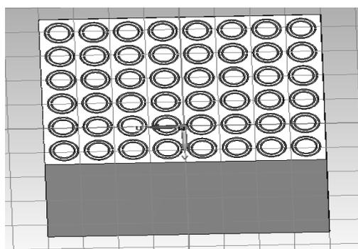
Fig.3 . Rectangular patch antenna with srr on substrate
