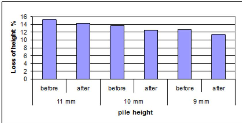
figure 1. Dynamic results of pile height loss
