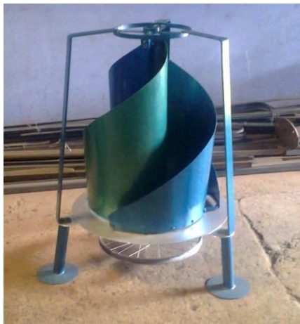
Figure 3: Involute spiral wind turbine blade model
