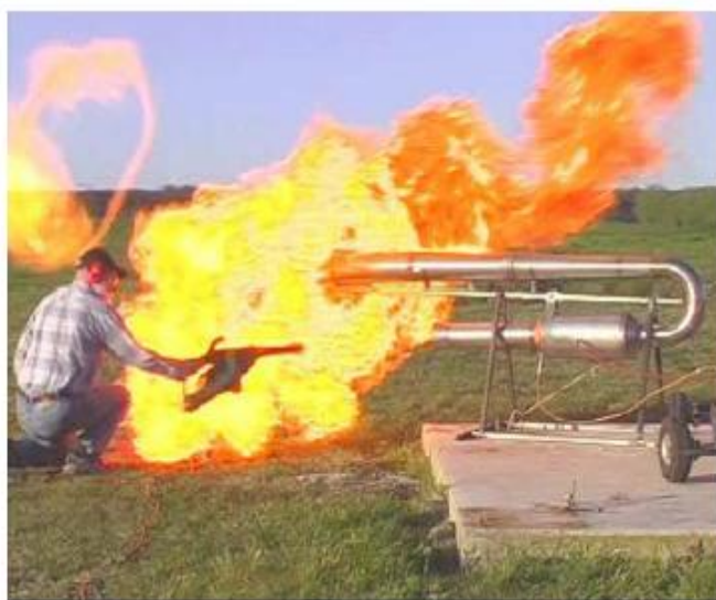
Figure Leaf blower air assist start (Simpson 2005)
