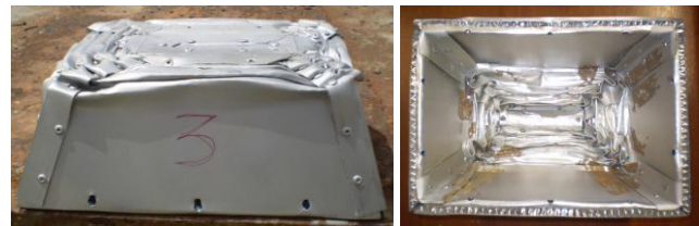
Figure 5: Impact attenuator after test: external and internal view.
