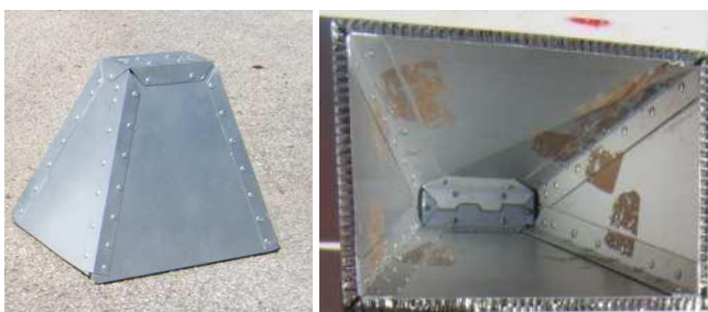
Figure 1: Impact attenuator: external and internal view.
