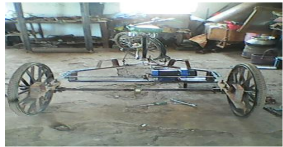
Fig. 4. Drive Train – Manual pedal retrofit three-wheeler with grid powered
