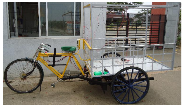
Fig 6: optimized solar powered cum manual driven load carrying three-wheeler rickshaw
