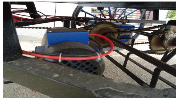
Fig. 5. Position of the motor with its sprockets & pulleys
