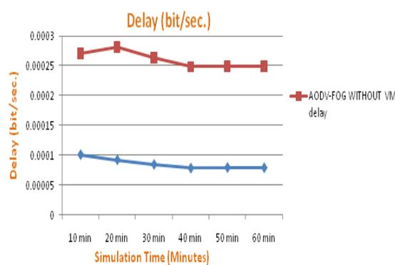
**Fig. 4 – Delay of fog computing with & without VM**
