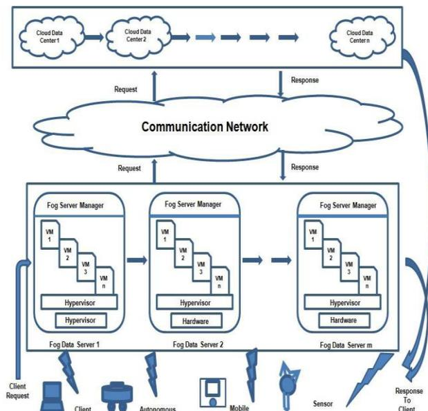
**Fig. 2 Three Layer Architecture for Resource Allocation in Cloud-Fog System**
