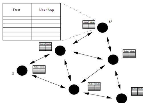
Figure 2. Proactive Routing Scheme
