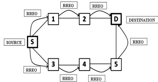
Figure 3. Route Request Reactive Routing
