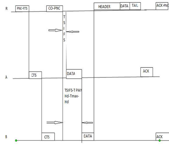
Figure 1: Packet exchanges in DMAC
