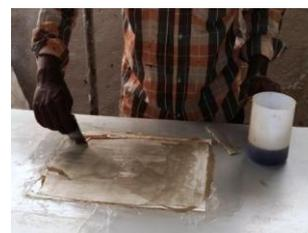
Fig.3 Preparation of Laminated Specimens. [4]
