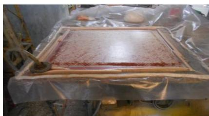
Fig. 5 Manufacture of Glass fibre laminate using Vacuum hand lay – up technique [9]
