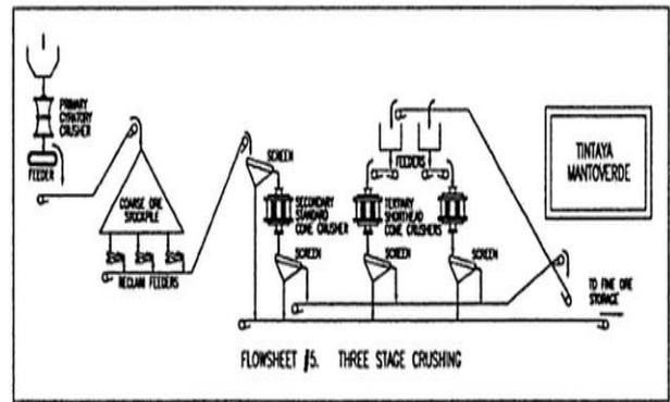
Fig.04 The Layout showing the crushing in the three stages crushing (Both Fine & Coarse Product)
