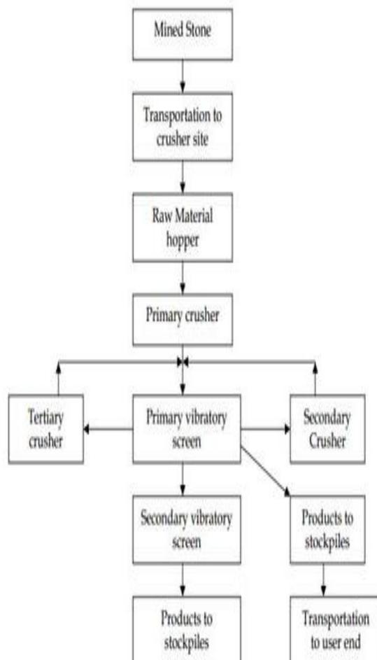
Fig. 05 Block diagram typical process of stone crushing plant
