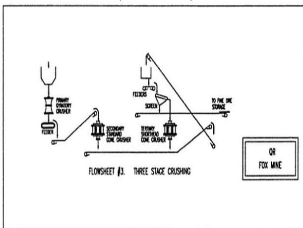
Fig. 03 The Layout showing the crushing in the three stages crushing. (Both Fine & Coarse Product)
