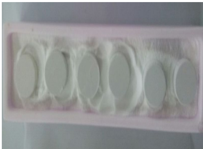
Figure 1: Pellets formed by hand press machine kept in the alumina boat for sintering process.
