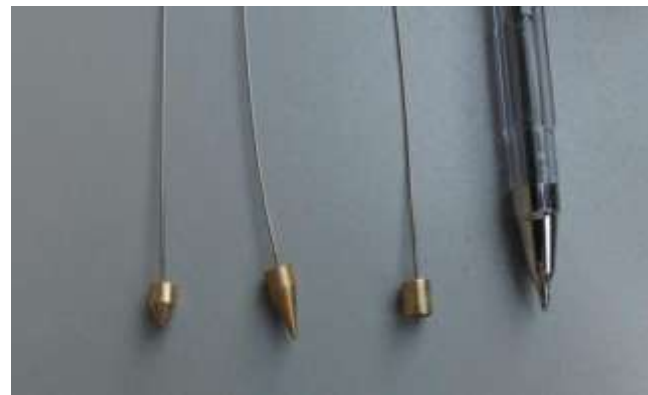
Fig.3. Conical and flat disk-shaped cavitators
