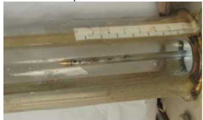
Fig.2. The model comprising of cylindrical body and a conical cavitator inside the test section
