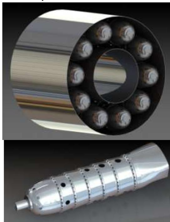
**Figure 4:** CAD model of combustor
