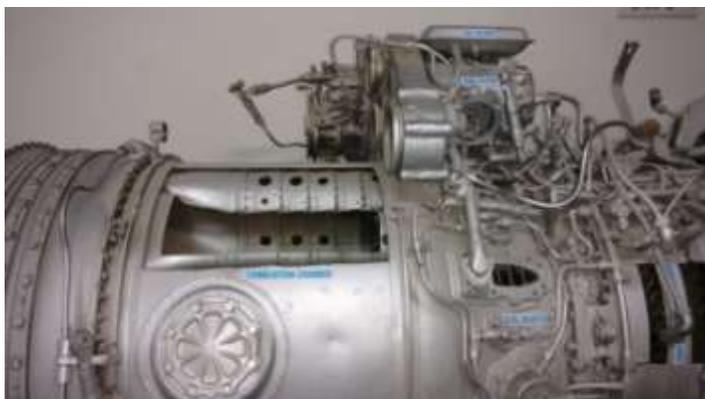
**Figure 1:** Cut-section of combustor (ACED, Propulsion Lab)
