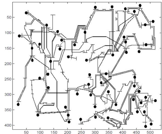
Fig. 20 Scaling of IEEE 118 bus system
