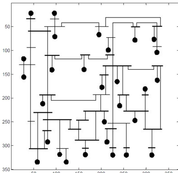
Fig. 18 Scaling of IEEE 39 bus system
