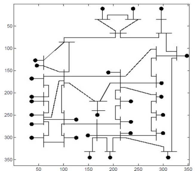
Fig. 16 Scaling of IEEE 30 bus system
