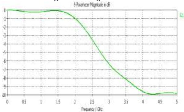
Fig. 2 Simulated Result of low pass filter
