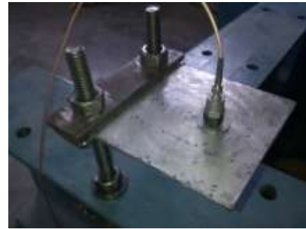
Fig.3 Plate fixed with CFFF condition
