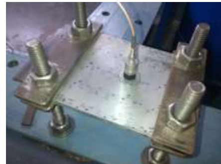
Fig.4 Plate fixed with CFFF condition
