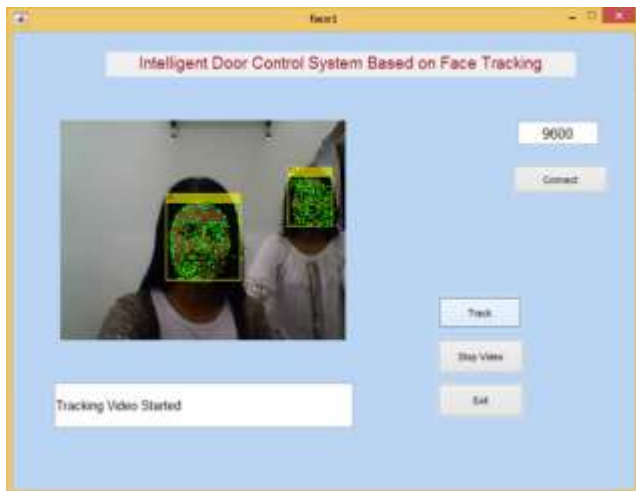
Fig.18. Matlab GUI result when the two persons are detected
