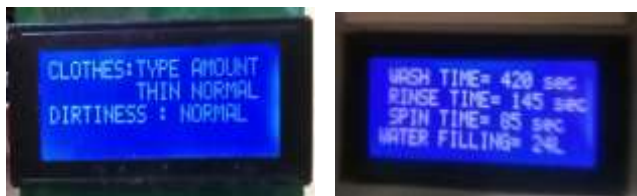
Fig19. Experimental Result for Thin Clothes
