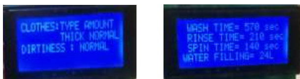
Fig20. Experimental Result for Thick Clothes
