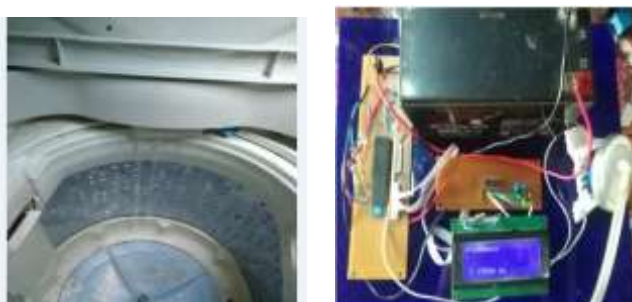
Fig11. Measuring frequency data by using controller depend on the water level into the tub
