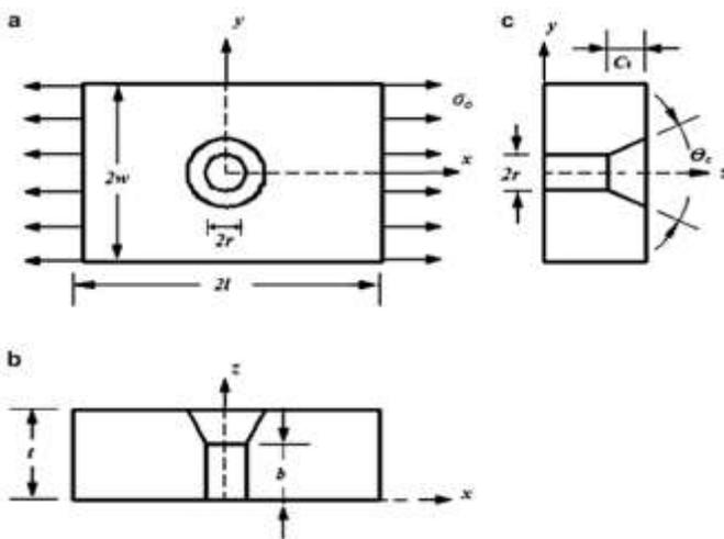
Figure 7: Configuration of Countersunk hole [8]
