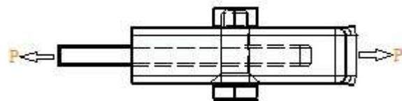
Figure 4: Bolted joint in Composite leaf spring
