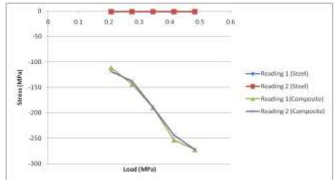
Figure 17: Graphical representation of Stress Results for Countersunk Bolted configuration
