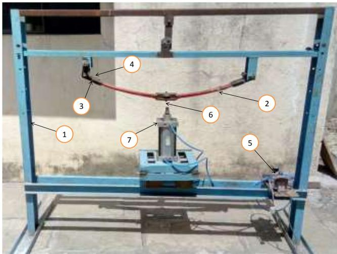
1. Frame, 2.Spring, 3.Strain gauges 4.Bolted Joint 5. Pneumatic circuit 6. Load cell 7. Screw Jack
