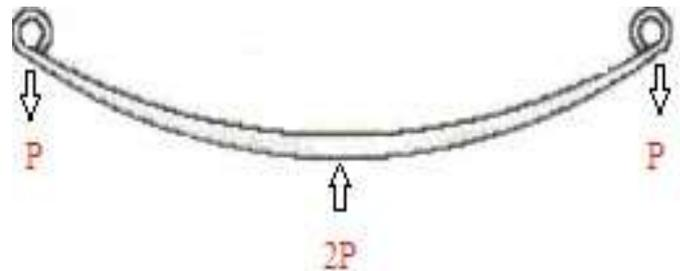
Figure 3: Forces acting on Composite leaf spring
