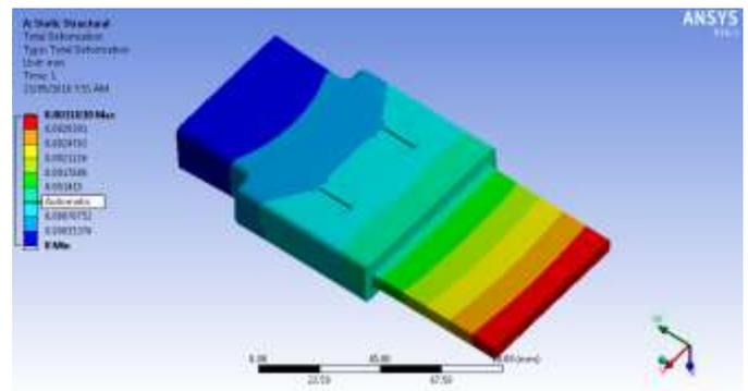
Figure 13: Total Deformation of Countersunk Bolted Joint
