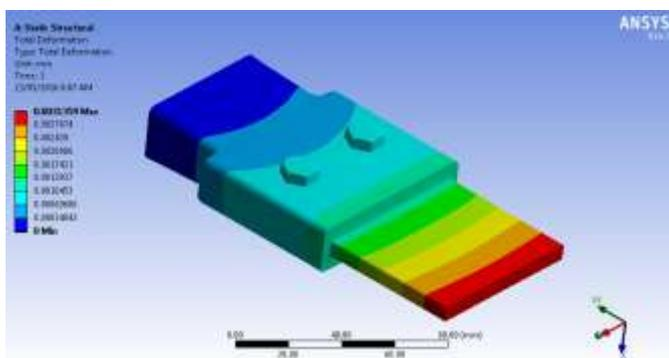
Figure 11: Total Deformation of protruded Bolted Joint
