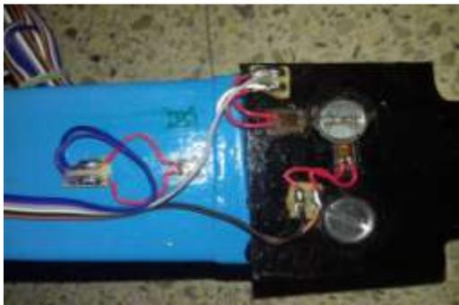
Fig.15.Mounting of Strain Gauges
