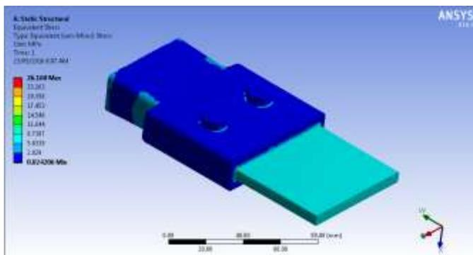
Figure 10: Equivalent Stress of Protruded Bolted Joint
