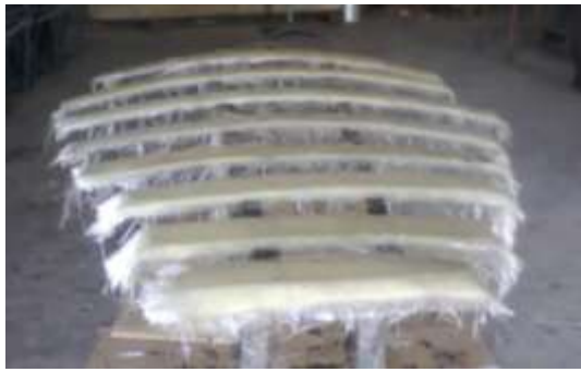
Fig 6 Placing of fiber layers over profile
